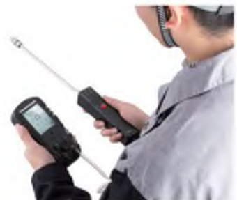
external pump gas detector
