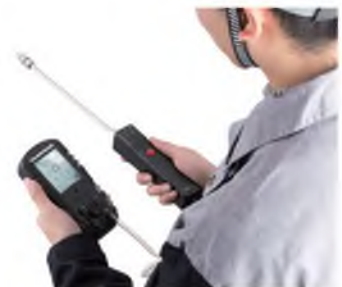
external pump gas detector
