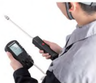
external pump gas detector
